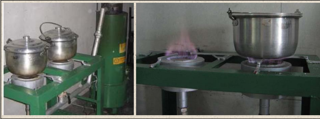
The two-burner rice husk gas stove - Philippines
