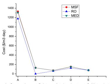
A= Construction cost, B=Intermediate loop heat cost, C=Water plant cost, D=Water plant contingency, E= Infall/Outfall 15
