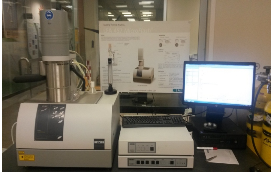
Laser Flash (LFA-457) Thermal Conductivity Measurement System
